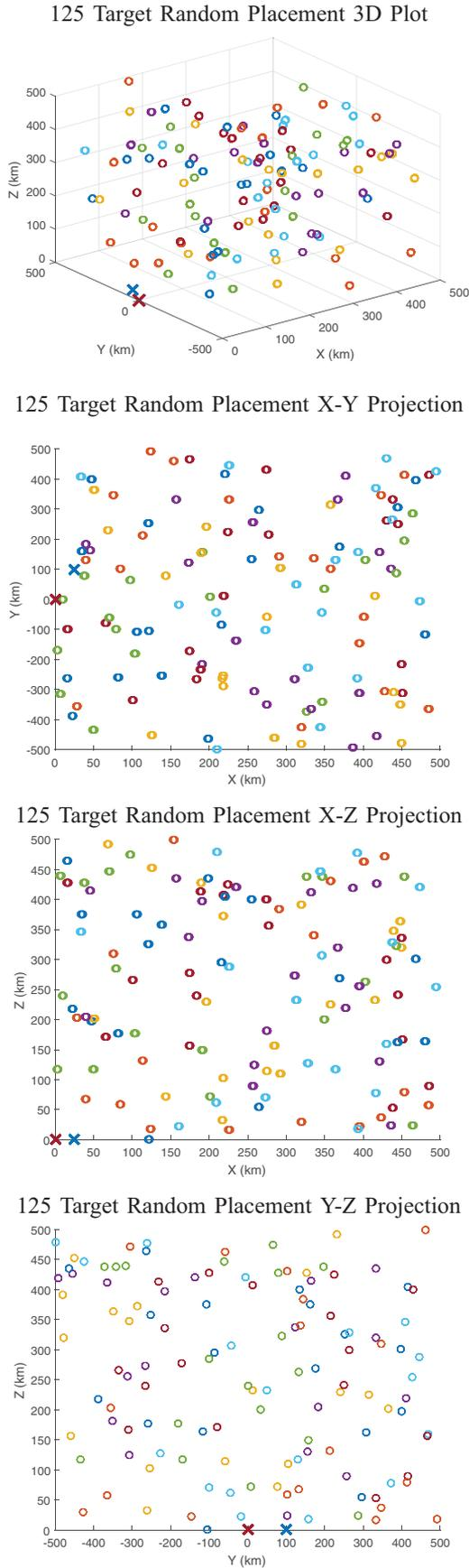
Figure 4. 125 random target layout with projections. The  $\times$  symbols represent sensors and the  $\circ$  symbols represent targets. (a) 3D plot. (b) X-Y projection. (c) X-Z projection. (d) Y-Z projection.
